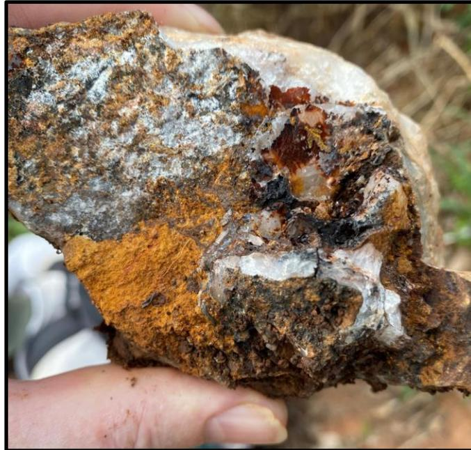
**Plate 9-12 Jagger Zone trench KTR010 with quartz veining, tourmaline and Fe oxides**
