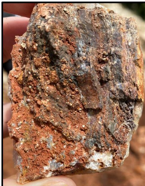
**Plate 9-17 Highly sheared ferruginous altered basalt**
